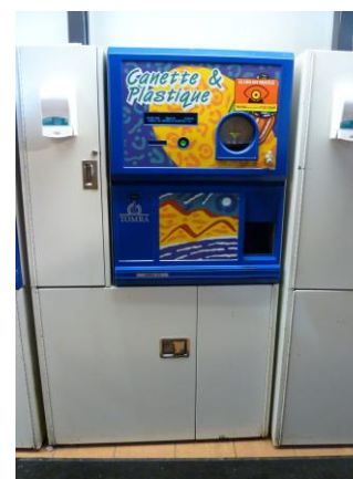
This machine takes plastic bottles and cans, sorts by bar code, and credits customers. See also P4
